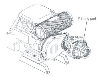
**l** Close the priming valve after priming. Failure to close the priming valve could cause the pump to lose prime or water to be pumped through the priming system.
